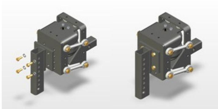
*Insert 4 bolts and torque to 55 ft-lbs not to exceed 100ft-lbs.*
